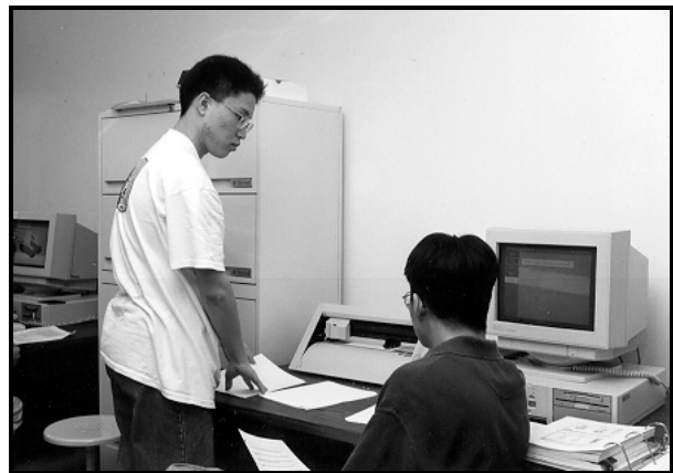
Figure 11. The students cut the slice outlines on adhesive paper using the JP System 5 rapid prototyping system.
