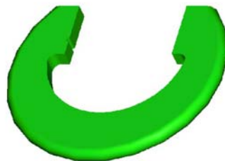
Figure 15 - A model of the gap gauge modeled using family tables.
