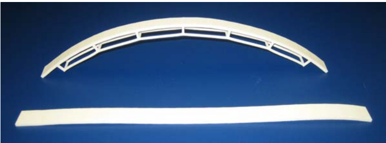
Figure 12. Arch prototype with and without lattice structure.
